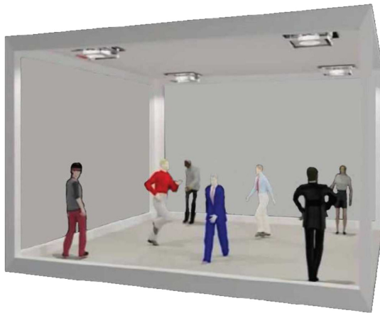
Fig. 3. Mobile users random mobility algorithm in an indoor dynamic VLC scenario for a standard room of dimensions 5 \times 5 \times 3 \text{ m}^3 .
